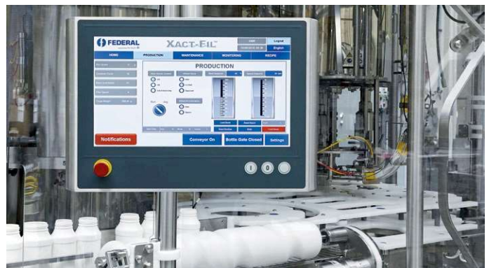
A Beckhoff CP3918 Control Panel with an 18.5-inch multi-touch screen serves as an advanced and intuitive user interface.
