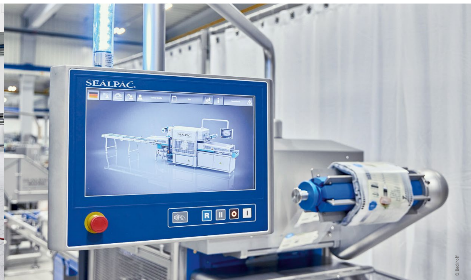
Controlled by PC-based control, the SEALPAC Traysealer A7max achieves a high processing capacity of up to 120 packages per minute.
