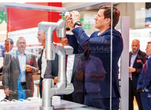
ATRO is a modular industrial robot platform that is fully integrated into TwinCAT and can be used to assemble optimal robot structures for different applications on an individual and flexible basis.
