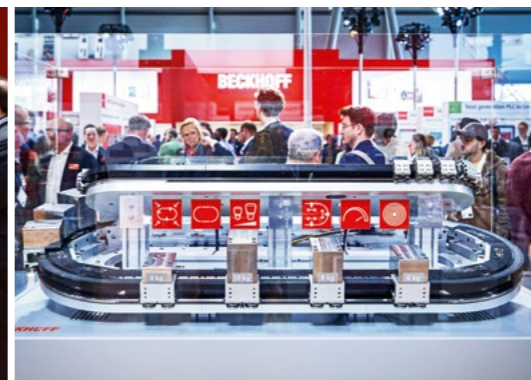
Beckhoff offers two intelligent handling systems that set new standards: XTS (shown here) for maximum freedom in one dimension and high dynamics, and XPlanar for contactless product handling with up to six degrees of freedom.
