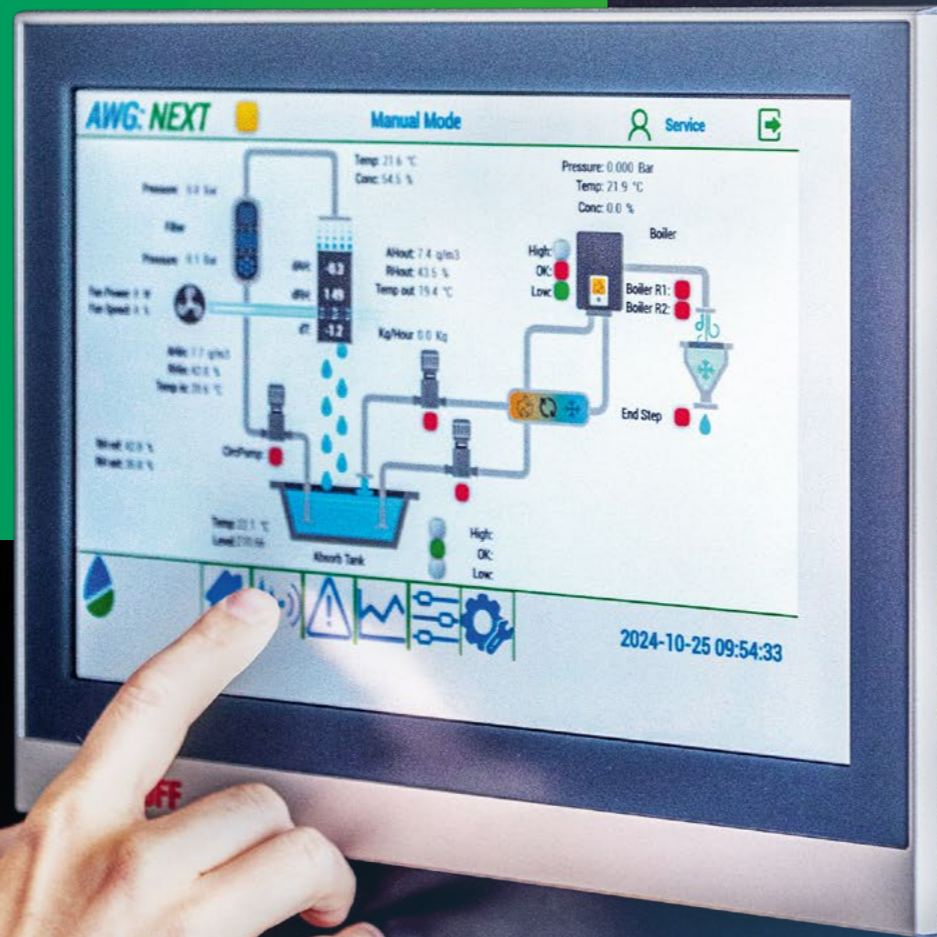
The dehumidifier parameters can be called up and adjusted on the control panel via the visualization implemented with TwinCAT HMI.
